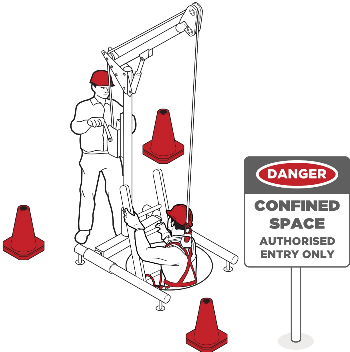
Figure 7 Standby person monitoring the confined space with rescue equipment and sign in place
